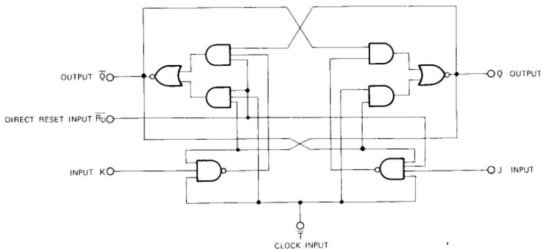
**DUAL J-K NEGATIVE EDGE-TRIGGERED FLIP FLOPS WITH RESET**
